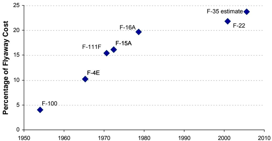
**Figure 3.2 - Increasing Complexity of Aircraft, as Expressed by Avionics Cost<sup>23</sup>**
